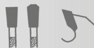
TCG teeth disc upper alternating bevel for laminate cutting
