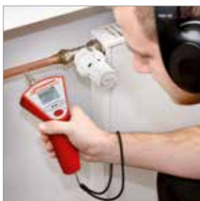
Acoustic leak detection of heating installations
