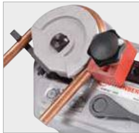
Forged aluminium former with bending radius display
